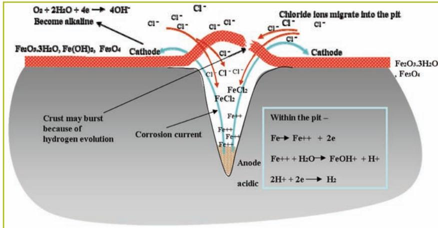
current leaves the surface and the cathode will become more OH<sup>-</sup> concentrated or more alkaline. Because of the physical condition in the deposit-covering pit, the positive Fe ions cannot be removed readily from the pit by the bulk solution and created the tendency to attract the negative ions.
