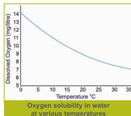
The presence of oxygen and carbon dioxide can affect directly the corrosion rate of mild steel in water. The effect of these dissolved gases must be taken into consideration when designing corrosion protection. It is important to maintain the water pH value at high level.
