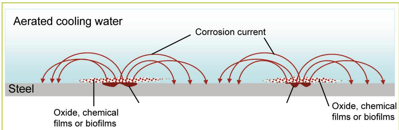
further in water to form ferrous hydroxides:
